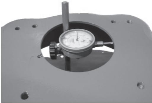
FIRST CHECK BELLHOUSING FOR BORE CONCENTRICITY. INSTALL MAGNETIC BASE TO FLYWHEEL OR PRESSURE PLATE, THEN INSTALL THE INDICATOR TO MEASURE THE BELLHOUSING BORE (SHOWN ABOVE). ROTATE THE CRANKSHAFT AND MARK DOWN THE INDICATOR READINGS (MARKING THE BELLHOUSING WORKS WELL). THE MAXIMUM OUT OF CONCENTRICITY IS .005".
