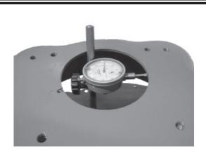
FIRST CHECK BELLHOUSING FOR BORE CONCENTRICITY. INSTALL MAGNETIC BASE TO FLYWHEEL OR PRESSURE PLATE, THEN INSTALL THE INDICATOR TO MEASURE THE BELLHOUSING BORE (SHOWN ABOVE). ROTATE THE CRANKSHAFT AND MARK DOWN THE INDICATOR READINGS (MARKING THE BELLHOUSING WORKS WELL). THE MAXIMUM OUT OF CONCENTRICITY IS .005".
