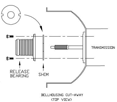
Centerforce recommends installing a new Ford Release Bearing/Slave assembly each time a new clutch is installed.
