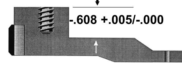
It is important to maintain the proper flywheel step specification. Failure to maintain the proper step specification may result in poor clutch performance, slipage, and/or improper release.
