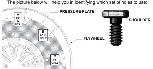
NOTE: 6 bolts are required to properly locate and fasten the pressure plate to the flywheel. Original equipment flywheels use (6) 5/16" shouldered bolts; bolt hole A & B (see above) to locate and retain the pressure plate. Some aftermarket flywheels may have a pattern aligning to the bolt holes A & C. The pressure plate may be bolted to such flywheels with shouldered 3/8" bolts in holes A & C.
