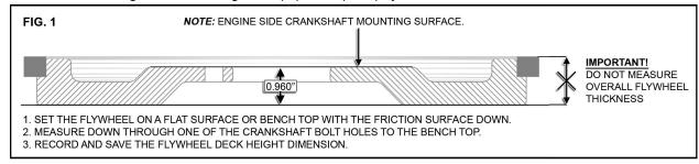
FIG 2 shows the O.E. clutch fork pivot ball height of 4.750" as measured from the engine block side of the Bellhousing plate (block saver) to the flat of the clutch fork pivot ball. If your flywheel deck height measures between 0.910" and 0.960", be sure your clutch fork pivot ball height is 4.750". If your flywheel deck height is less than 0.910" you will need to adjust the clutch fork pivot ball height to accommodate the thinner flywheel as follows:
