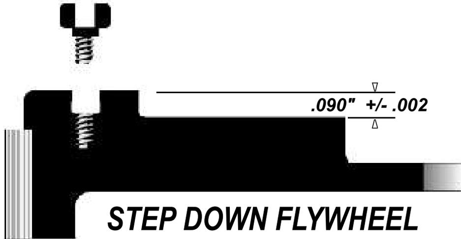
It is important to maintain the proper flywheel step specification. Failure to maintain the proper step specification may result in poor clutch performance, slippage, and/or improper release.
