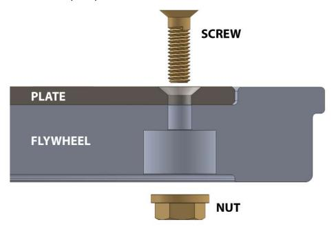
Screwed on friction surface plate installation as follows:
