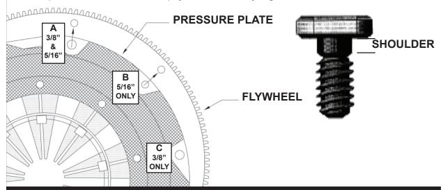
NOTE: 6 bolts are required to properly locate and fasten the pressure plate to the flywheel. Original equipment flywheels use (6) 5/16" shouldered bolts; bolt hole A & B (see above) to locate and retain the pressure plate. Some aftermarket flywheels may have a pattern aligning to the bolt holes A & C. The pressure plate may be bolted to such flywheels with shouldered 3/8" bolts in holes A & C.
