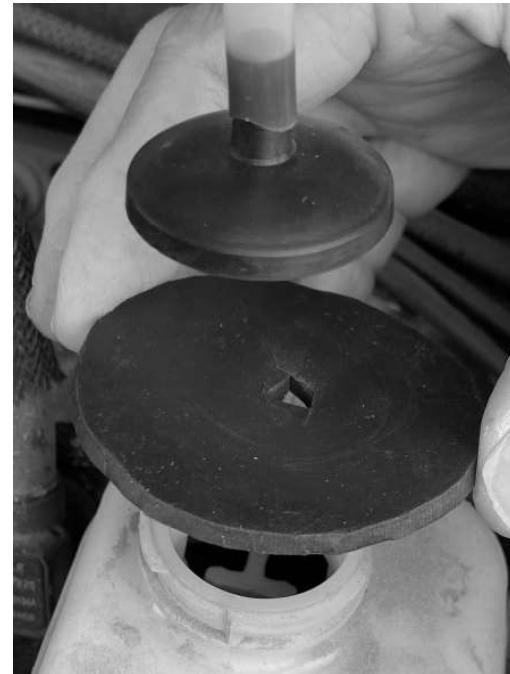
**Note:** It's common for small air bubbles to remain aerated within the clutch fluid for several hours. The clutch vacuum bleed procedure may need to be repeated after the vehicle sits overnight.
